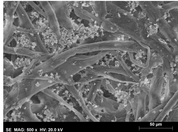
Figure 6. SEM image of the top side of paper sample (500x).
