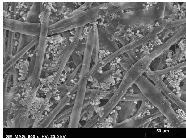
Figure 7. SEM image of the bottom side of paper sample (500x).
